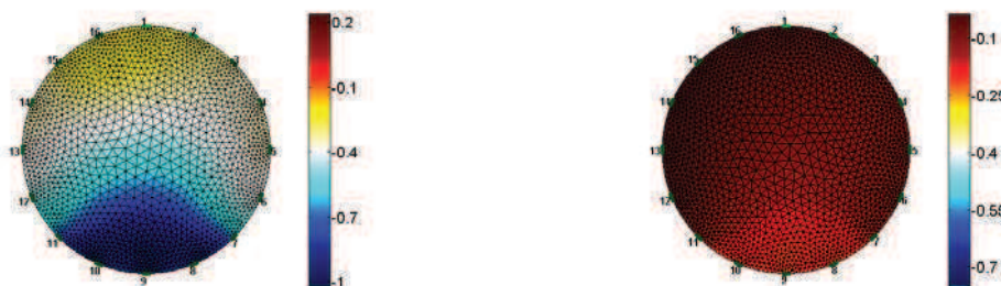
Figure 1 – Average glass beads concentration profiles for flow rates of 12 (left) and 52 m 3 /h (right).
